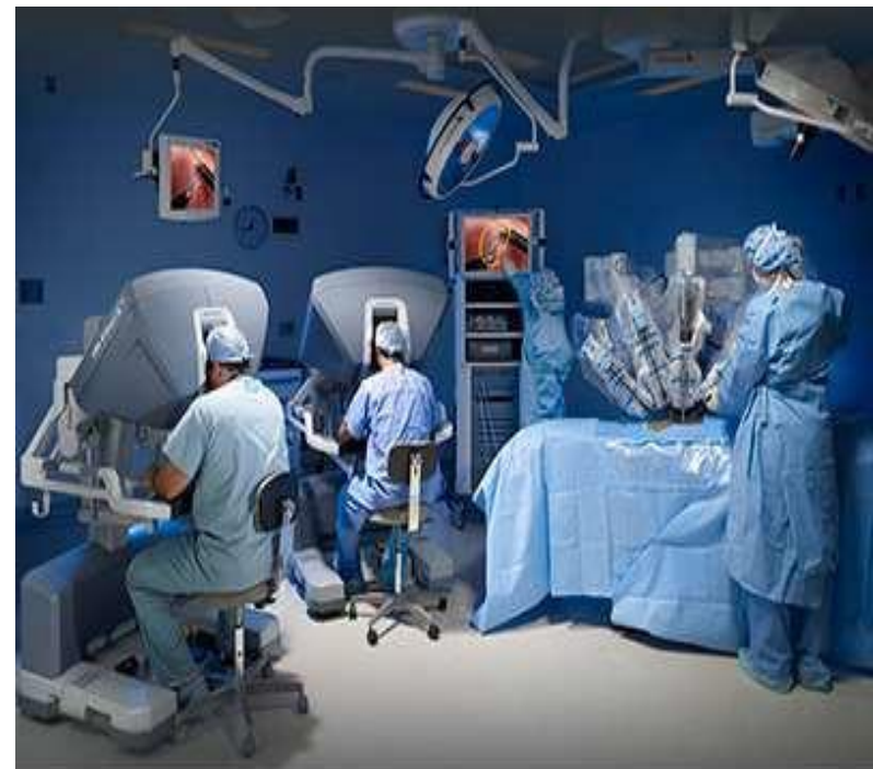
Teleoperated robot-assisted surgical system for minimally invasive procedures. (Credit: Intuitive Surgical, Inc.)
